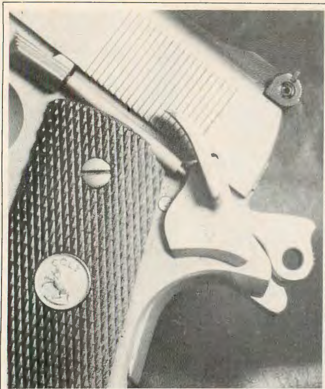
Extended grip safety and Colt Commander hammer eliminate "hammer bite syndrome." Swenson safety is worth expense as it allows gun to be put into action more rapidly. Note pinned (deactivated) grip safety.
